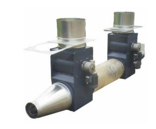
STYROMETER mixing station to ensure an accurate mixing of EPS recycled material and new beads just before the blockmould. Either directly into the blockmould or to the blockmould feeding silo. Also for mixing EPP materials before the pre-pressurizing tank.
